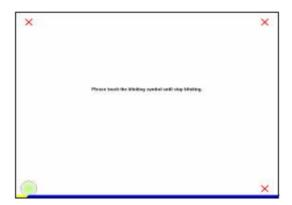
Touch the blinking symbol on panel until beep or stop blinking.
