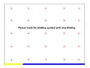
Touch the blinking symbol on panel until beep or stop blinking.
